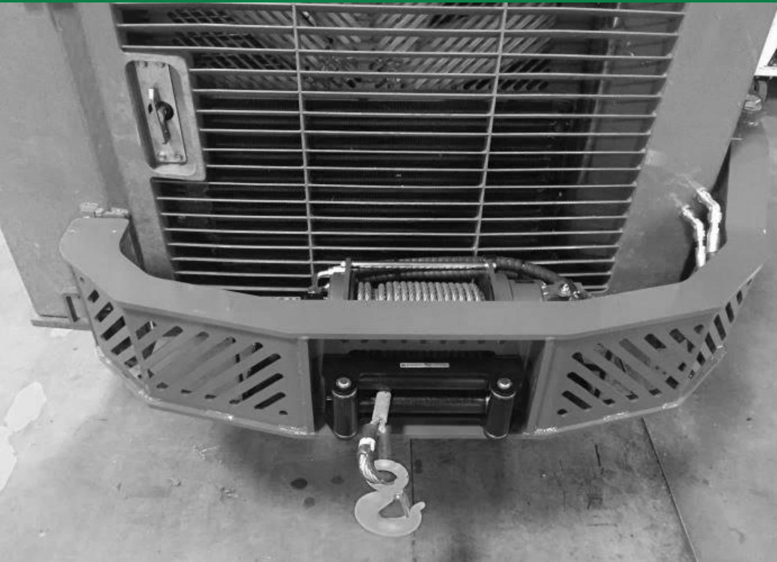
Winch and rear bumper can be supplied as an additional option. It's a Warn Hydraulic Winch with up to 15,000 lbs / 6,800kg pulling force. Controlled within the cab from the keypad.
